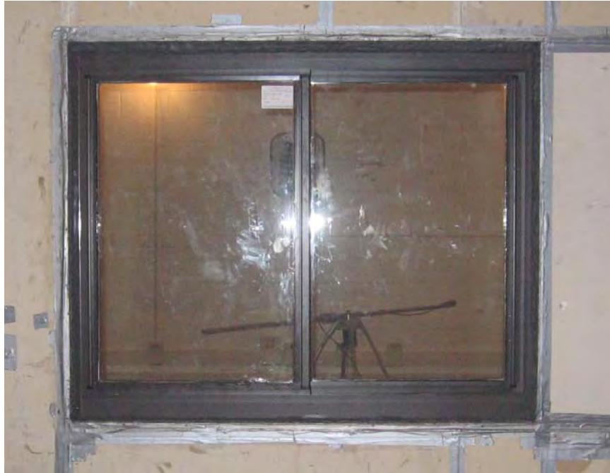
Receive Room View of Installed Specimen
